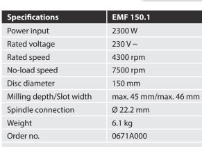
Supplied in a case incl. 2 diamond blades Premium (concrete) and assembly tools
